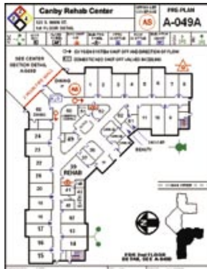
This diagram shows key building details such as walls, doors, sprinklers, hydrants and FDCs.
